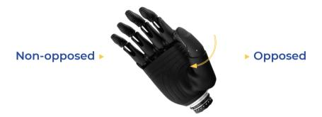
To move the thumb from the opposed to the **non-opposed position**, please hold the thumb at its base with your free hand and push it steadily outwards in a controlled manner.
