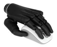
This grip can be used to show a number from 1 to 5 using the fingers. Pulses of the opening signal increase the count, pulses of the closing signal decrease it. Count can be reset to 0 by holding a closing signal.
