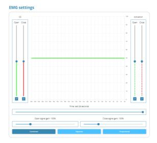
o Separate - in this option, both muscle signals (Flexion and Extension) are shown on the separate graphs
